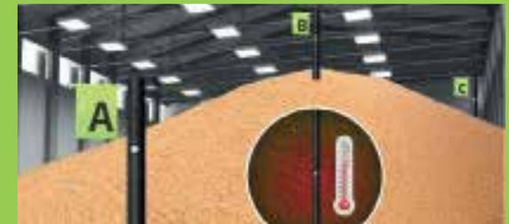
Measured values are transmitted wirelessly and are stored by the system, enabling the user to access stored data. If critical conditions are detected, the system automatically triggers an alarm via text message or e-mail.
