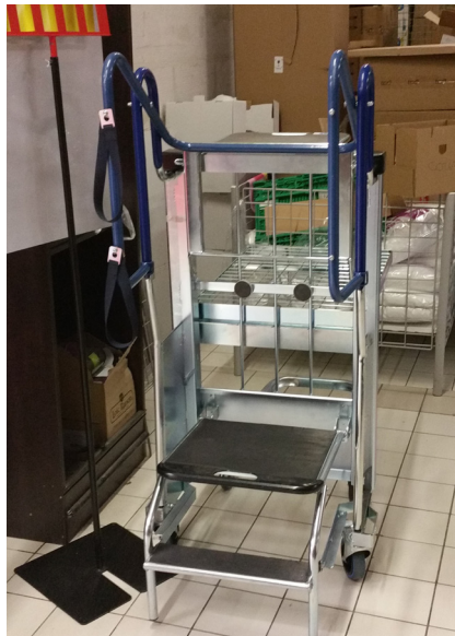
The equipment is useful for customers and the replenishment of goods weighing less than 15 kilograms. The tool reduces strain on shoulders by providing a static support for the parcel.
